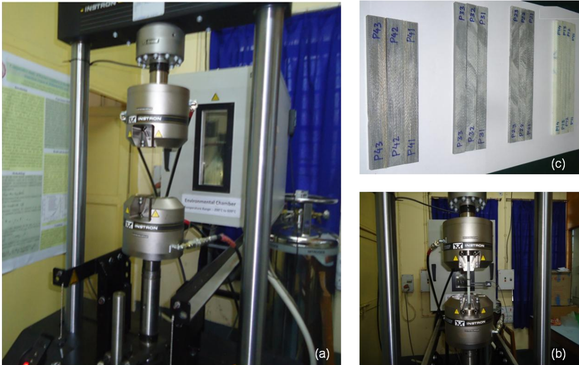
Figure 2.6 (a) INSTRON 8801, (b) tensile test setup, (c) test samples
