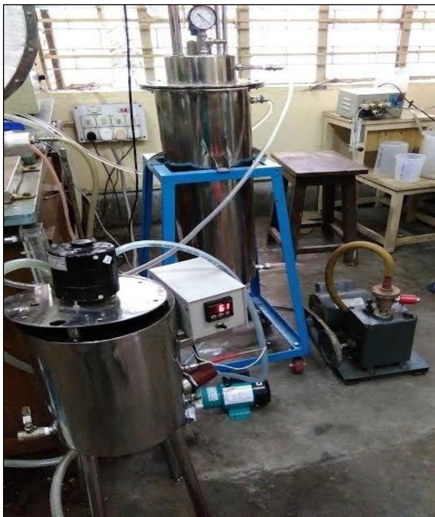
Fig3: The set up for Wiped film evaporator
